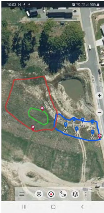
Photo 3. Green line = B grade stockpile to be removed, red line = extent of subgrade cut, blue line = fill site
