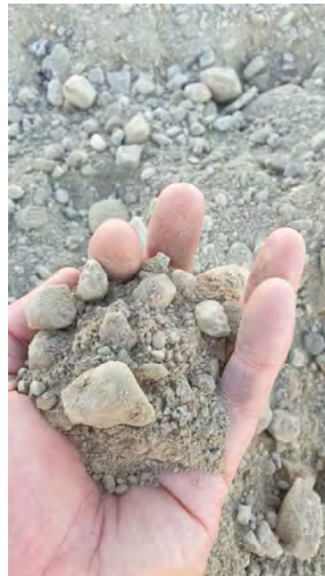
Photo 7. Proposed site won fill material (Gravelly SAND)
