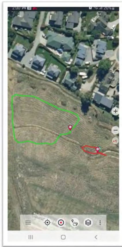
Figure 1. Greenline = extent of subgrade strip, Redline = small road alignment fill area
